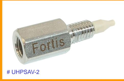
The Fortis™ UHPLC Filter (figure 3) is a pre-column filter that is suitable for operation under UHPLC conditions. It contains a 0.2um porous frit and is designed to possess minimal dead volume, this ensures that it does not significantly contribute to any band broadening.
