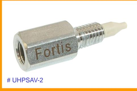
The Fortis™ UHPLC Filter (figure 3) is a pre-column filter that is suitable for operation under UHPLC conditions. It contains a 0.2um porous frit and is designed to possess minimal dead volume, this ensures that it does not significantly contribute to any band broadening.
