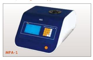
MPA-1 Digital Melting Point Apparatus is integrated with photoelectric detection, digital temperature display and other technologies, boasts automatic display of initial and final melts and other functions. In the temperature system, linearly calibrated platinum resistor is used as the detection device, offer efficient and accurate test process and results.
