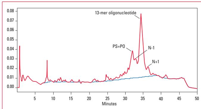
Although the customer's current column, widely considered an industry standard for oligonucleotide separations, provided similar chromatography; the performance declines dramatically after approximately 5 injections. Subsequent work shows the TSKgel DNA NPR column has continued to provide consistent results beyond 50 injections.
