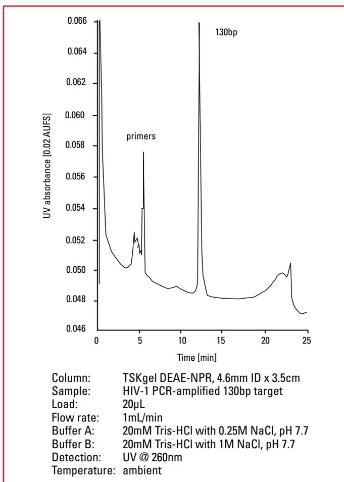
Figure 9. Detection of HIV-1 PCR-Amplified 130-bp target using a TSKgel DEAE-NPR Column
