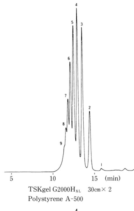
Fig. 13 Separation of polystyrene oligomer by TSKgel H<sub>XL</sub> type columns
