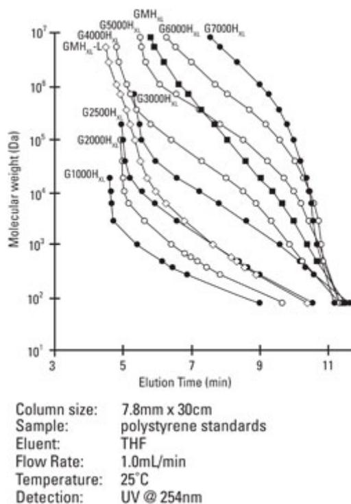
**Fig. 3 TSKgel H<sub>XL</sub> calibration curves**
