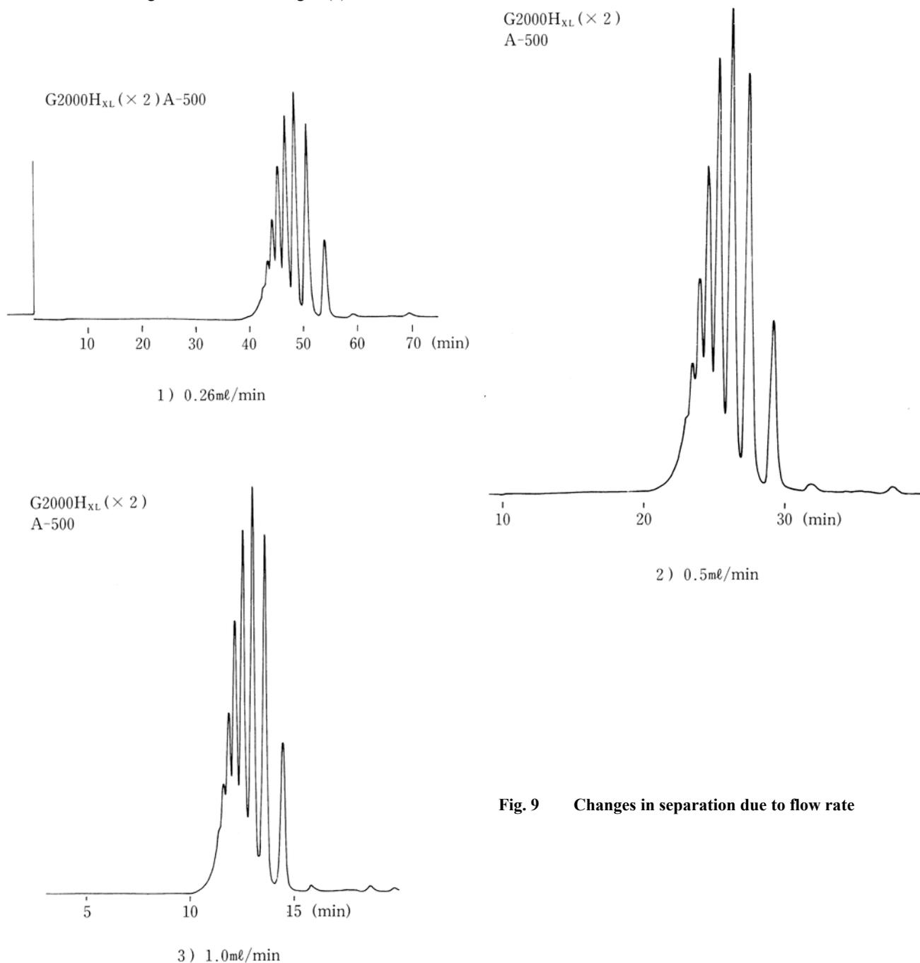
**Fig. 9 Changes in separation due to flow rate**
