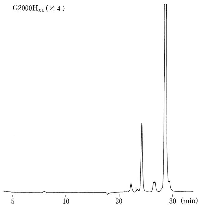
Fig. 18 Separation of Epikote 828
