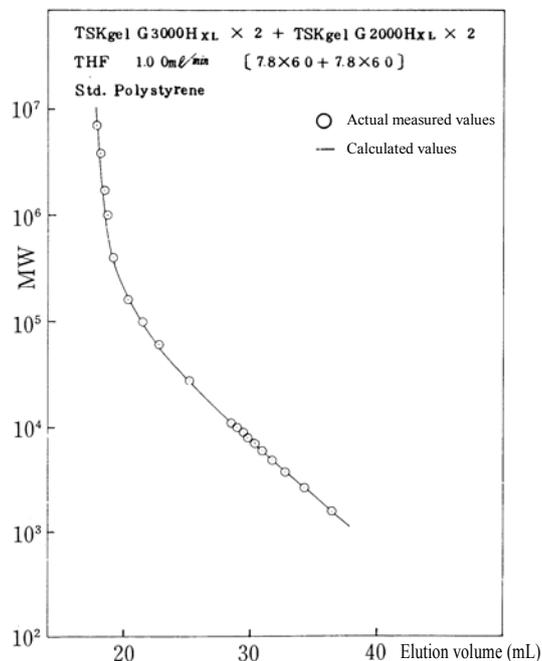
**Fig. 8 Calibration curve of TSKgel G2000H<sub>XL</sub> + TSKgel G3000H<sub>XL</sub>**
