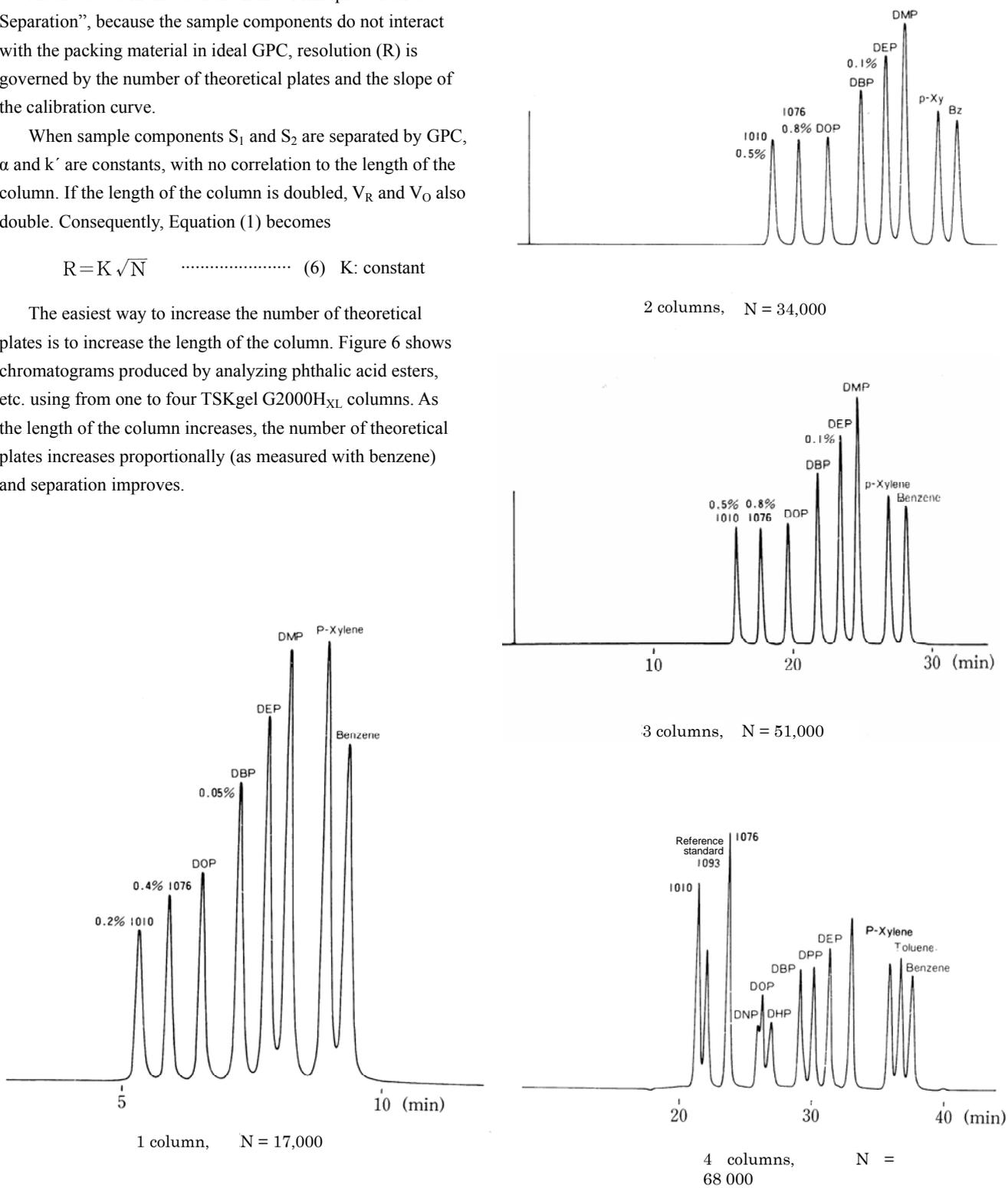
Fig. 6 Separation of phthalic acid esters by TSKgel G2000H<sub>XL</sub>
