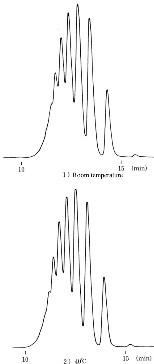
**Fig. 11 Effects of column temperature on separation**
