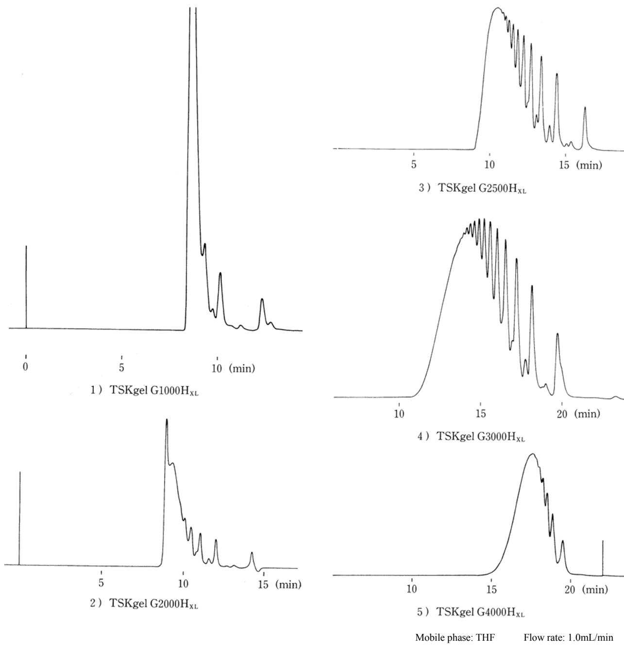
**Fig. 4** Separation of Epikote 1004 by TSKgel G1000H<sub>XL</sub> through TSKgel G4000H<sub>XL</sub> columns
