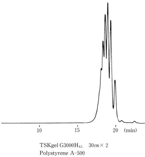
Fig. 13 Continued Separation of polystyrene oligomer by TSKgel H<sub>XL</sub> type columns
