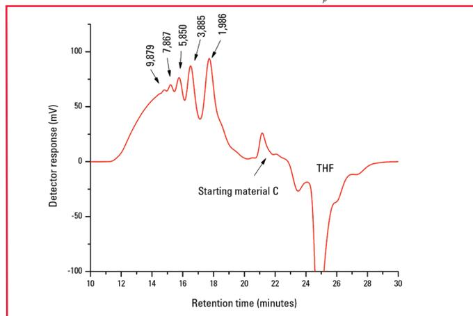
**Figure 3.** SEC analysis of PEG-B as monitored by RI. Numbers on graph represent polystyrene relative peak-average molar mass  $M_p$  values of each mode.
