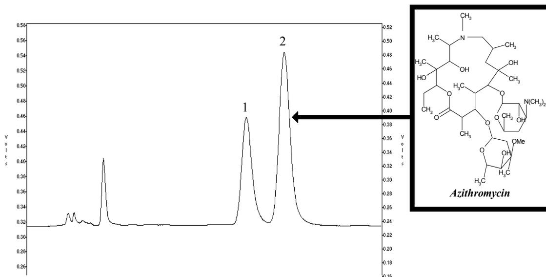
**LC Conditions:** Column, ZirChrom®-PBD, 150 x 4.6 mm i.d.; Flow Rate, 1.0 ml/min.; Mobile Phase, 29/71 acetonitrile/14 mM potassium phosphate monobasic at pH 11; Column Temperature = ambient; Detector, amperometric electrochemical; Injection volume, 50 microliters; Sample concentration, 5 micrograms/ml. Solutes: 1 = azaerythromycin, 2 = azithromycin.
